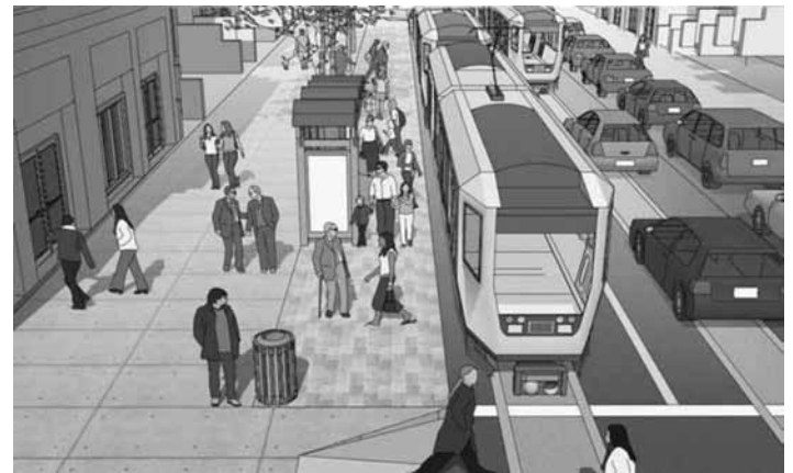
Rendering of proposed 9 foot bulb at Carl and Cole. (Image courtesy of San Francisco Planning Department, City Design.)
